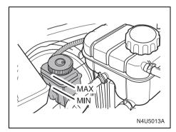
To check the fluid level, look on the side of the reservoir. If the fluid level is between the MIN and the MAX marks on the reservoir, the fluid level is correct. The reservoir is located near the back of the engine compartment on the driver's side of the vehicle. See "Engine Compartment Overview" in this section for more information on location.
